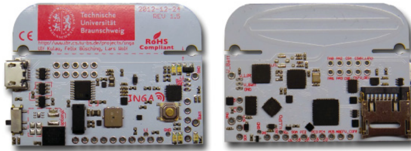
Fig. 2. Prototype of the undervolting-capable wireless sensor node with two independent and scalable voltage paths.
