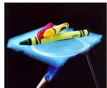
Figure 3: The aerogel plate isolates
