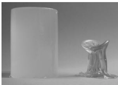
Figure 4: Hydrogel (left) and shrunken hydrogel after air drying (right) Source: Pakowski, Z. Drying of Nanoporous and Nanostructured Materials. In Proceedings of the 14th International Drying Symposium (IDS2004), Sao Paulo, Brazil, Vol. A; 2004; pp 69–88.
